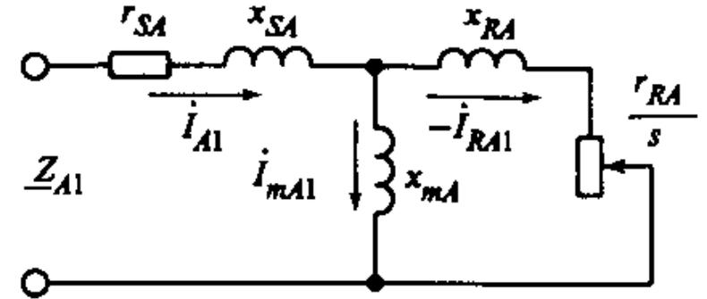
$$P_{\text{ЭМ1}} = P_{\text{ЭМА1}} + P_{\text{ЭМВ1}} = I_{RA1}^2 \frac{r_{RA}}{s} + I_{RB1}^2 \frac{r_{RB}}{s}$$
